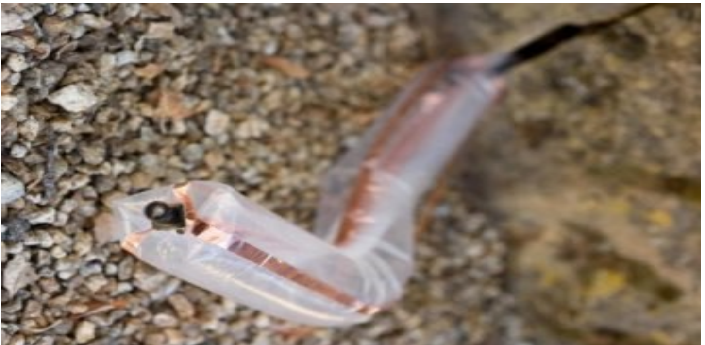
The vinebot is tube of soft material that grows in one direction.
