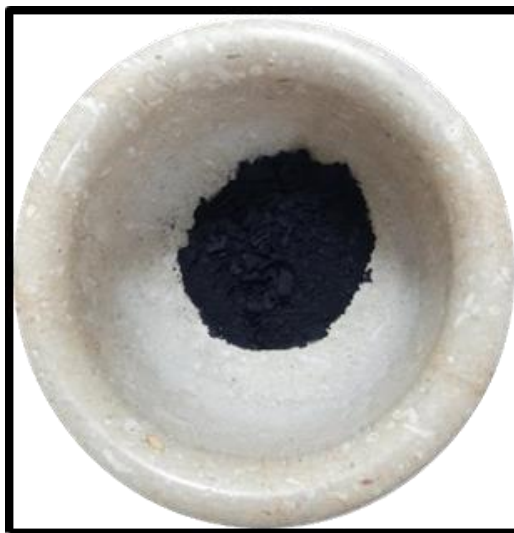
Figure 1. Superparamagnetic iron oxide nanoparticles coated with a naturally occurring biopolymer.
