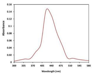
Figure 1. UV-Vis Spectra of Biosynthesized Silver Nanocomposite.
